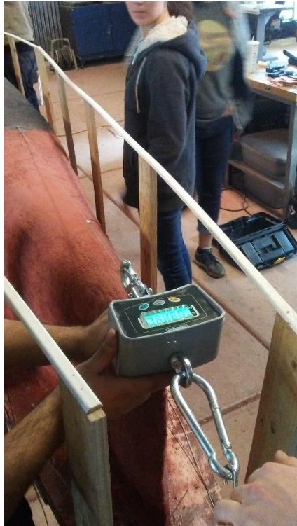
PHOTO 7 – Post-tensioning system with turn buckle and strain gage to monitor tension
