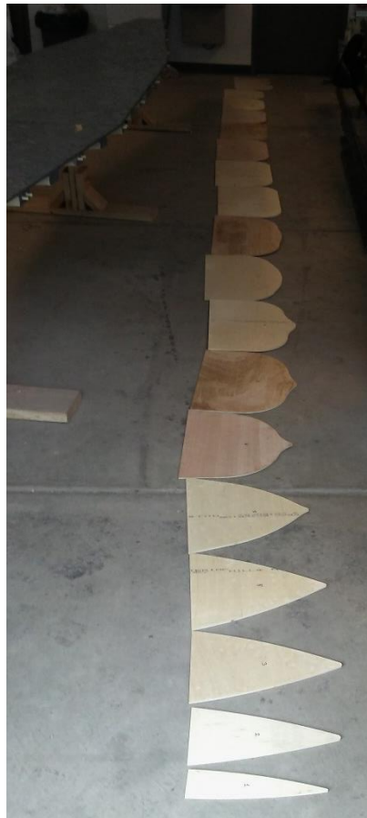
PHOTO 2 – Full cross section progression laid out post waterjet cutting
