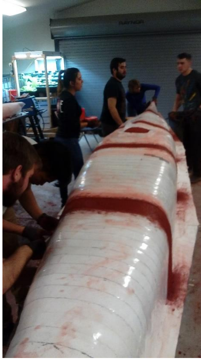
PHOTO 1 – Applying finishing mix to the rib cut outs on the mold
