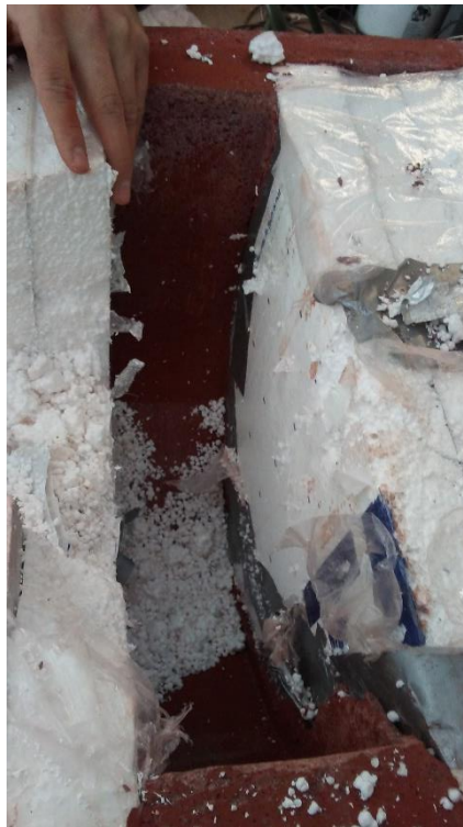
PHOTO 8 – Removing the first mold section to make room for the entire form removal
