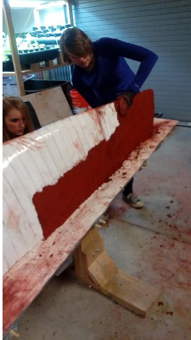
PHOTO 3 – Application of finishing mix fabricated tiles
