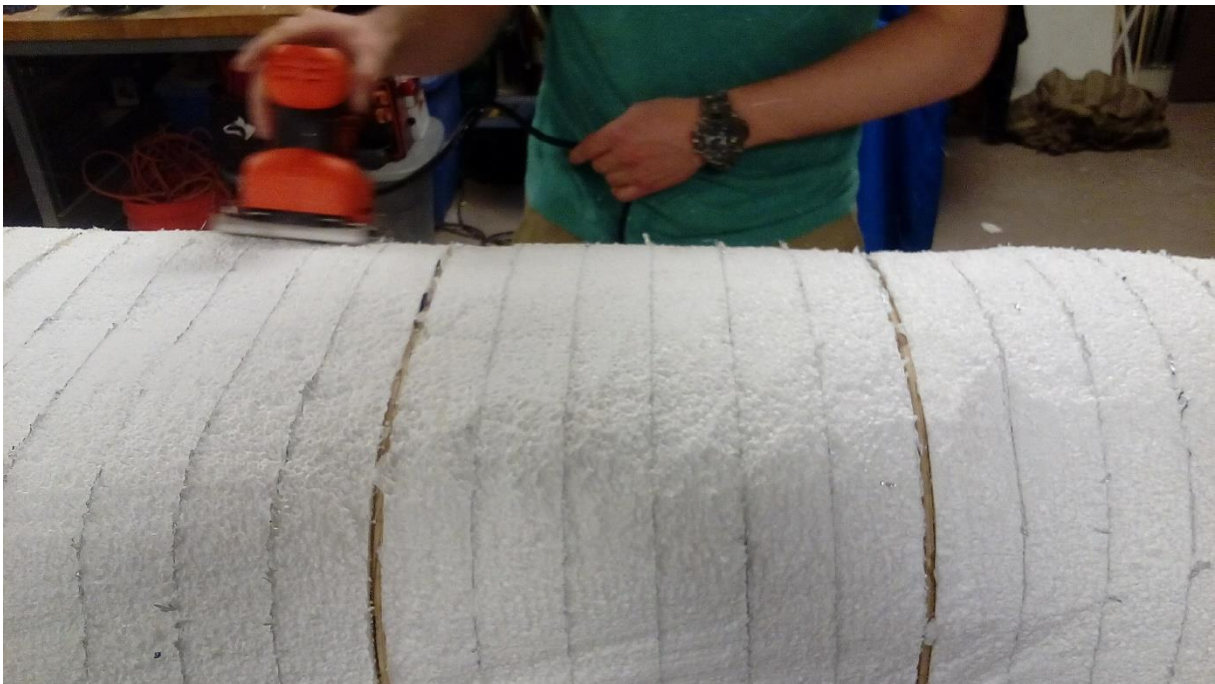
PHOTO 6 – Palm sanding the foam to be even with the cross-section design
