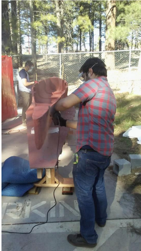
PHOTO 5 – Grinding and sanding down excess outer layer thickness
