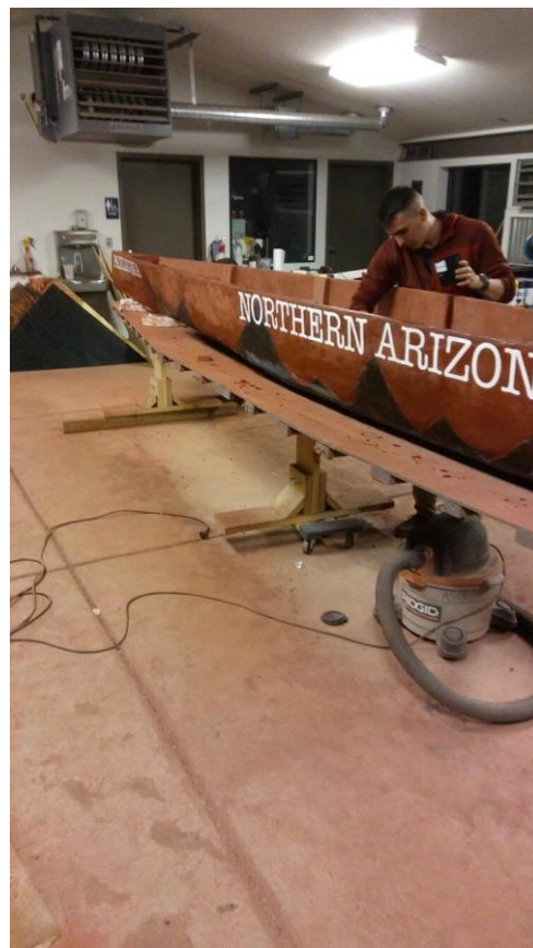
PHOTO 8 – Applying final seal coat
