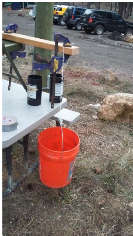
PHOTO 4 – Testing tensile strength of the mesh reinforcement
