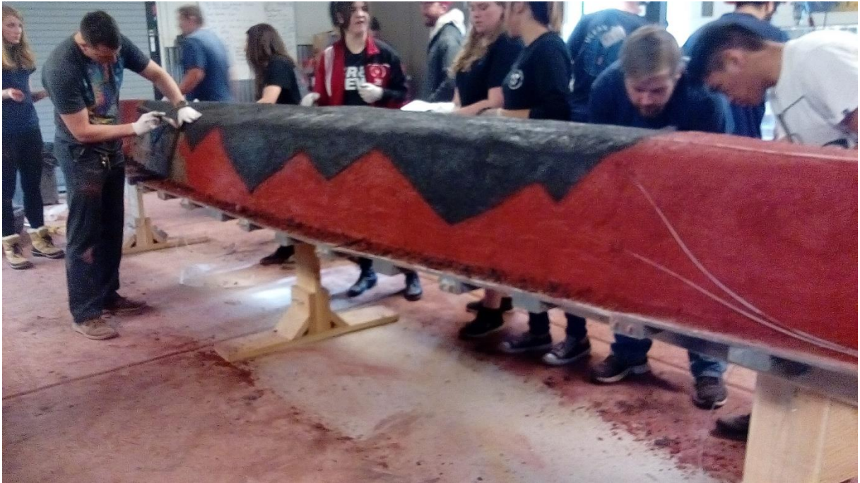
PHOTO 5 – Placement of two colored finishing to achieve a mountain peak look
