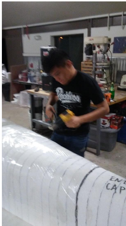
PHOTO 8 – Using heat gun to get the shrink wrap to form to the mold
