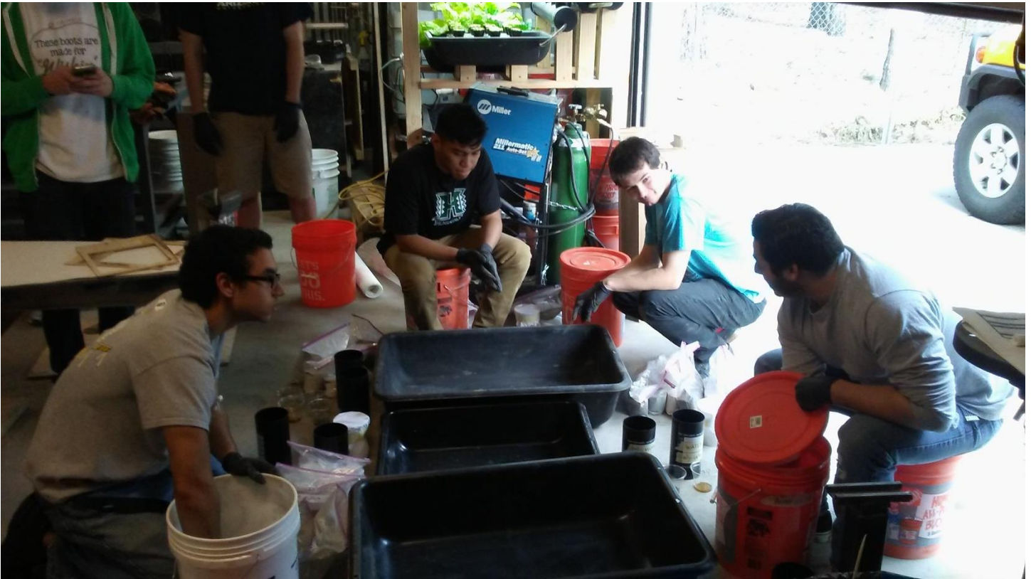
PHOTO 3 – Preparing cementitious materials and aggregate for hand mixing in tub
